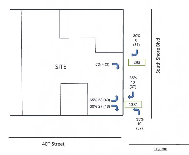
Figure 1 – Turning Movement Worksheet Wellington South Project # 22-130
