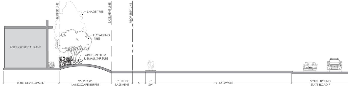
**A R.O.W BUFFER SECTION** SCALE: 1" = 10'-0"
