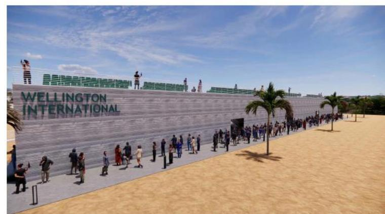
The stadium seating will be located around the main International Arena within the center of the venue. The structure is approximately 20 feet tall and 272 feet long. It will feature 13 rows and 1,554 permanent seats with a powder-coated guardrail. Seating will be hunter green to match the branding of the showgrounds. The open-air structure will have a cladding around the base of the metal structure with a pedestrian pathway underneath, enhancing the look of the structure.
