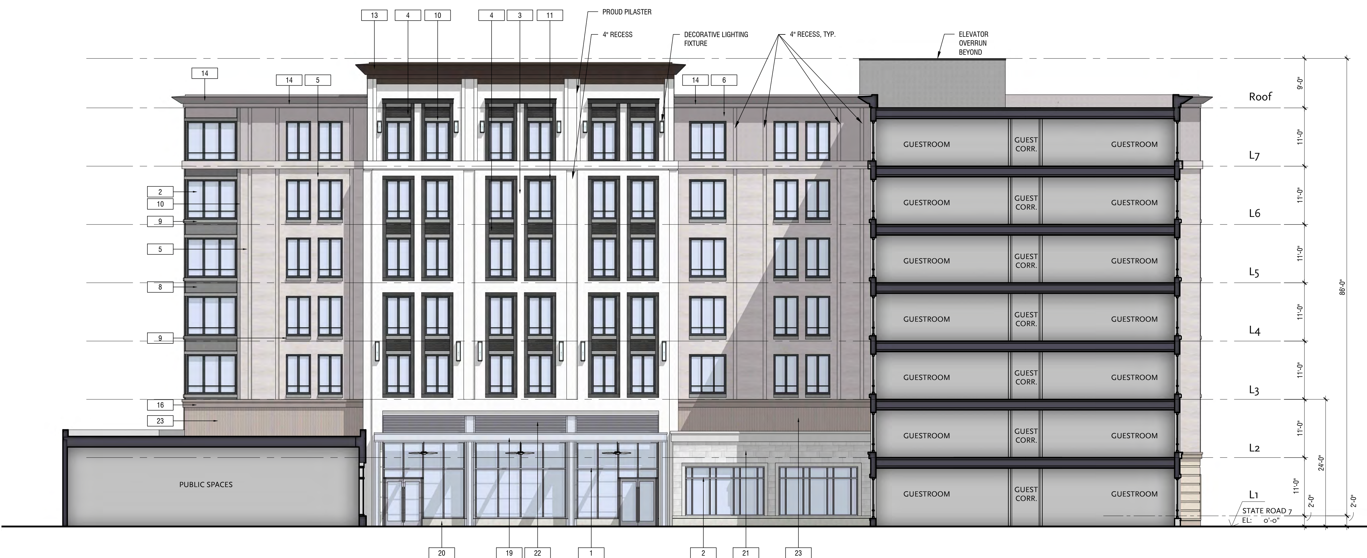
2 WEST ELEVATION - COURT SECTION SCALE: 3/32" = 1'-0"
