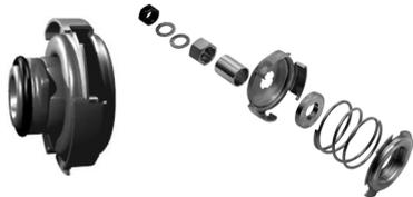
The pump shaft is connected to the motor shaft through a left thread and tight fit. The shaft cannot be dismantled.
