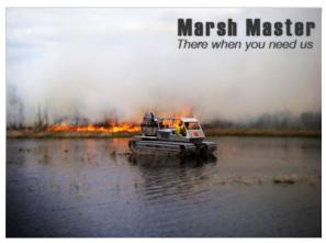
The MM-2 FF marsh buggy is designed for fire fighting and controlled burning in wetland environments. It incorporates the use of 55 gallon water tanks built into each pontoon, a hydraulically driven water pump, and an in-cab LED water level indicator. The fire pump is rigged with a suction hose and strainer that can be dropped into any water source for quick tank replenishment. The flow rate on the pump is approximately 22 gpm.
