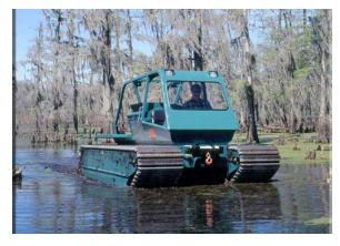
The **Marsh Master** is a tracked amphibious craft that can be used for a myriad of task. It has attachments for mowing, herbicide application, backhoes, anchor setting, and a geoprobe for soil sampling. The ground pressure of a Marsh Master is less then 2 lbs PSI, a human as a ground pressure in excess of 2.5 PSI
