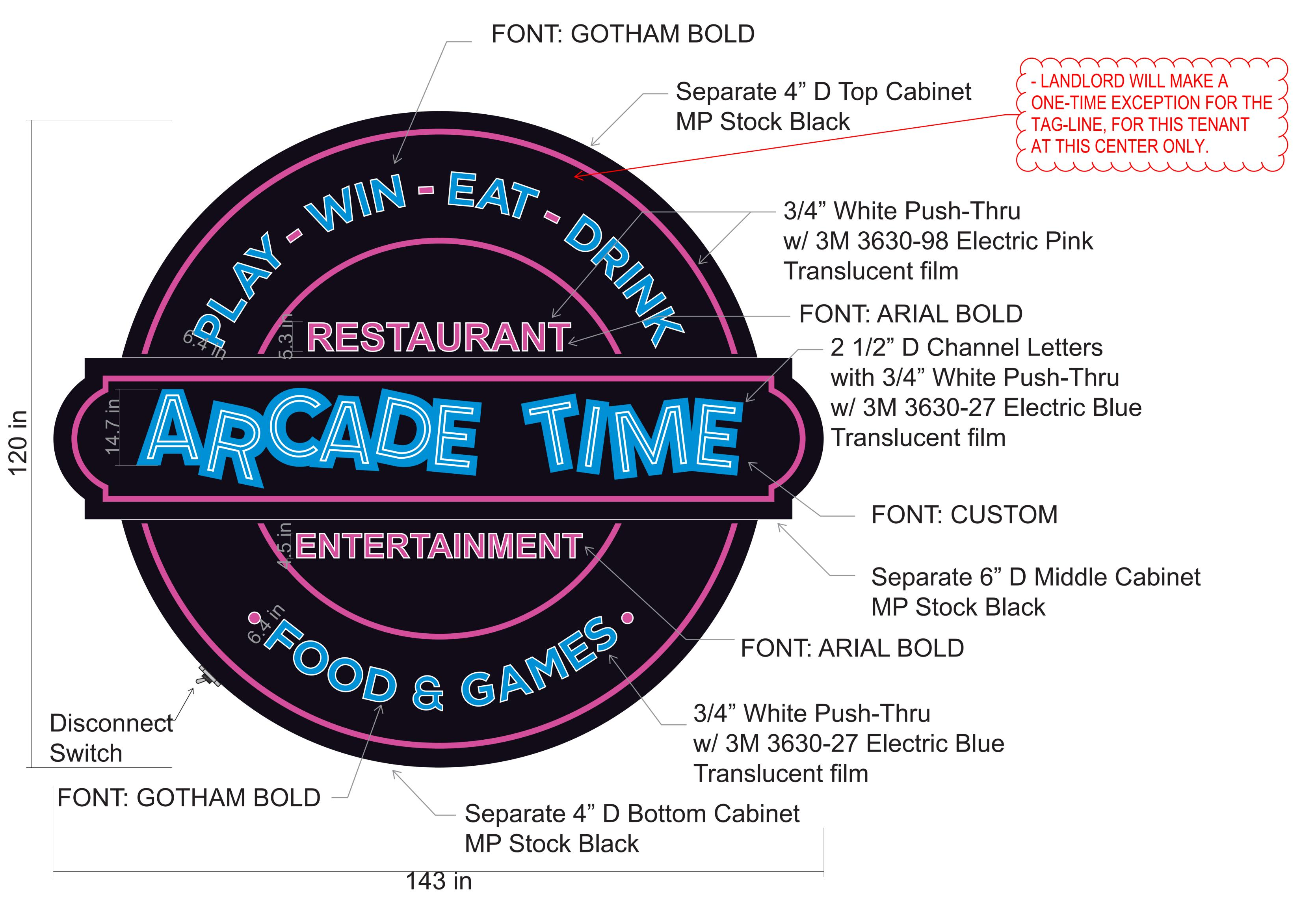
Separate 4" D Bottom Cabinet \_\_\_\_\_ MP Stock Black 3/4" White Push-Thru w/ 3M 3630-98 Electric Pink Translucent film 2 1/2" D Channel Letters with 3/4" White Push-Thru w/ 3M 3630-27 Electric Blue Translucent film Separate 6" D Cabinet – MP Stock Black Separate 4" D Bottom Cabinet MP Stock Black
