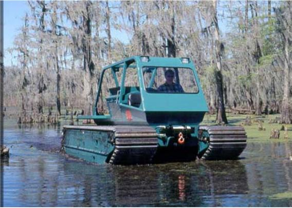
The **Marsh Master** is a tracked amphibious craft that can be used for a myriad of task. It has attachments for mowing, herbicide application, backhoes, anchor setting, and a geoprobe for soil sampling. The ground pressure of a Marsh Master is less then 2 lbs PSI, a human as a ground pressure in excess of 2.5 PSI
