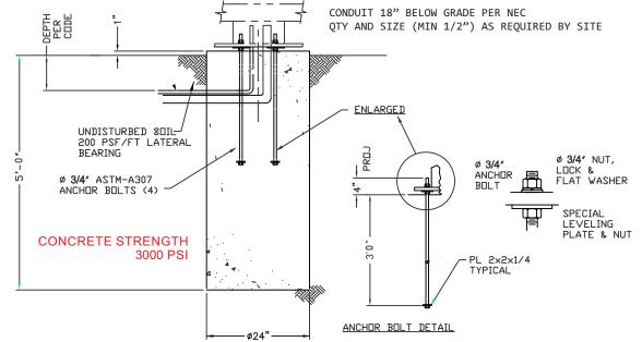
Visual inspection indicates 2,000 P.S.F. for which footings are designed. If a bearing capacity of less than 2,000 P.S.F. is encountered at site, the engineer shall be notified before proceeding with work.
