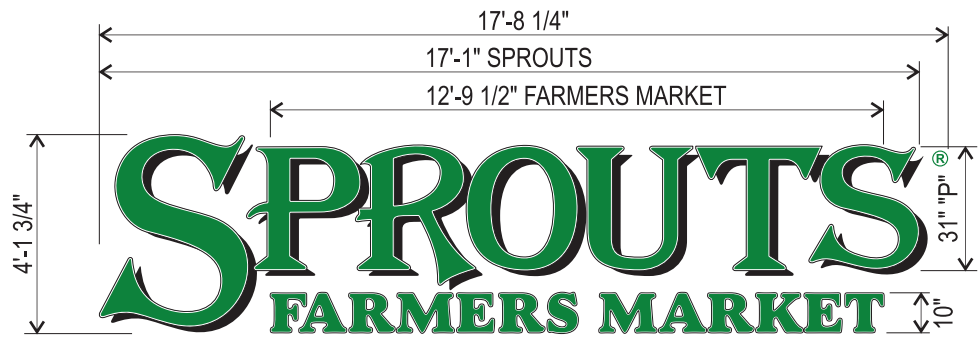
48" CHANNEL LETTERS SCALE: 1/4"=1'-0" AREA = 68.3 SQ. FT SFMLM48SFMG
