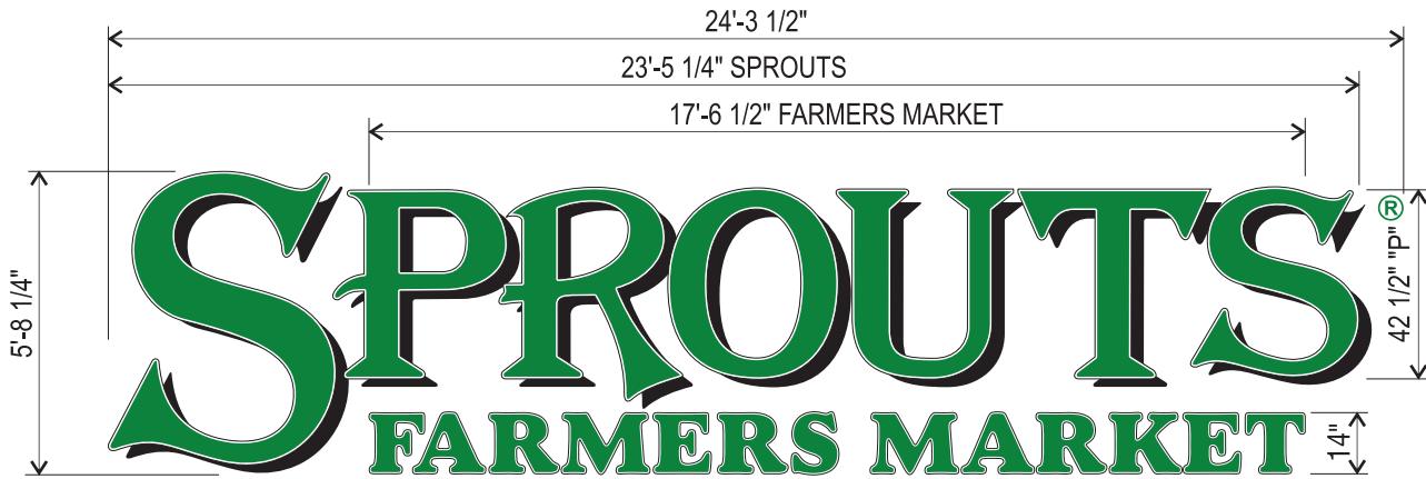
66" CHANNEL LETTERS SCALE: 1/4"=1'-0" AREA = 128.9 SQ. FT SFMLM66SFMG
