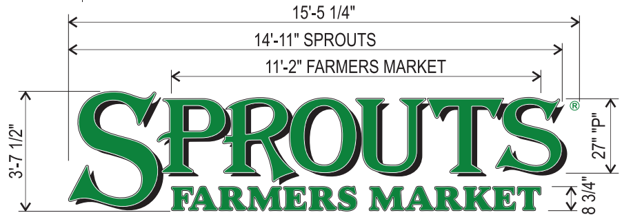
42" CHANNEL LETTERS SCALE: 1/4"=1'-0" AREA = 52.2 SQ. FT SFMLM42SFMG
