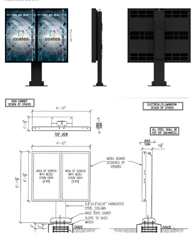
The other signs are two (2) digital "preview" menu board signs with a proposed height of 49 inches, length of 29 inches, sign area of 8.88 square feet and one (1) panel as illustrated below.
