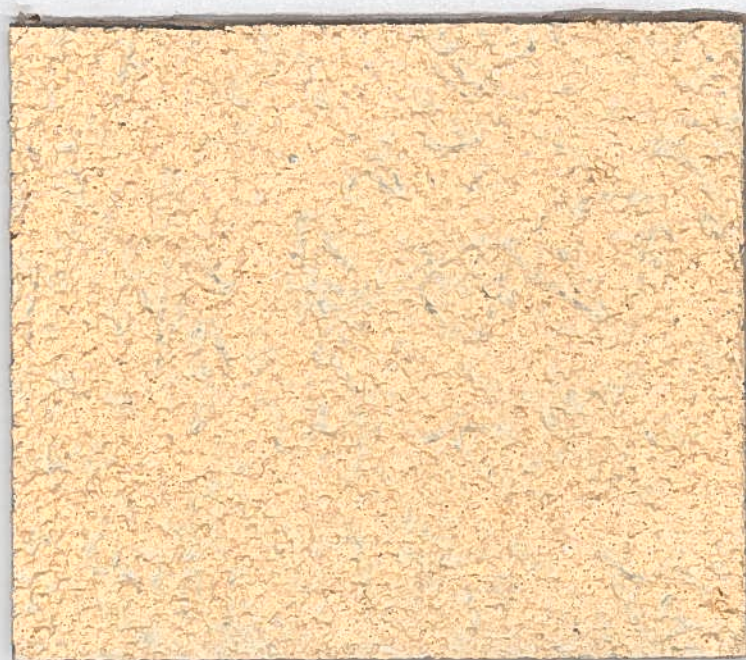
STUCCO & EIFS (K9 RESORTS CUSTOM CREAM COLOR WITH A SANDPEBBLE FINE FINISH TEXTURE)
