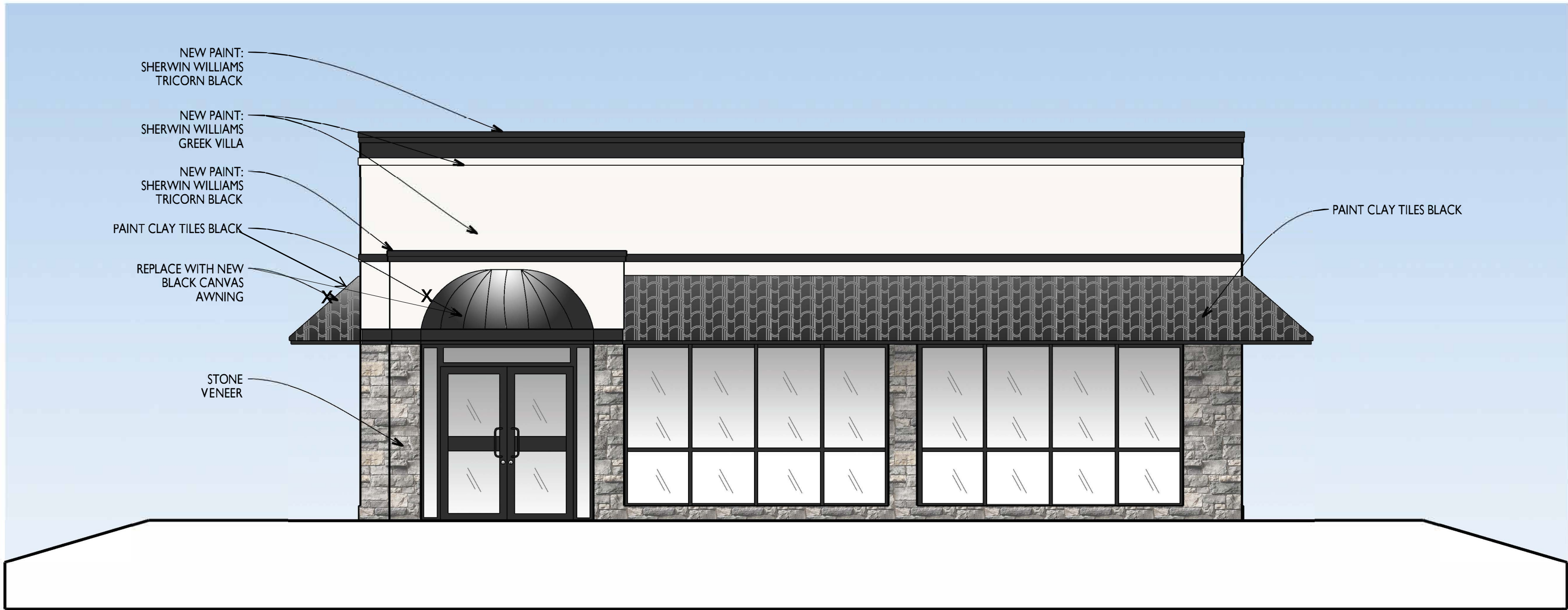
B A5 PROPOSED BUILDING ELEVATION WEST ELEVATION SCALE: 1/4"=1'-0"
