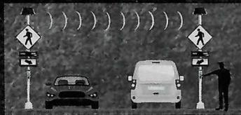
Wireless communication provides easy installation. No boring under roads!
